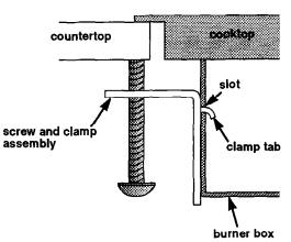
Insert one clamp tab through each slot located on sides of the burner
